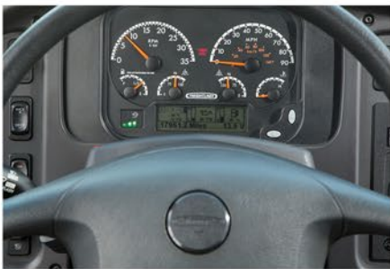
A non-reflective instrument panel with easy-to-read and LED-backlit gauges
