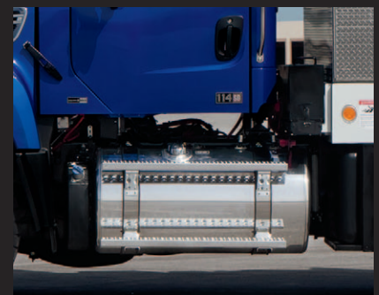
Fuel and DEF tank packaging for ease of body upfit.
