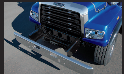
Tilt hood with radiator-mounted stationary grille and front frame extension.
