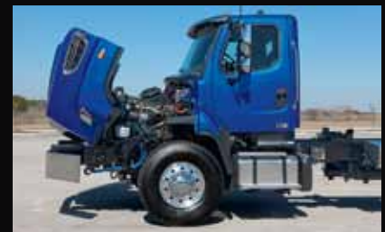
Full tilt hood for easy engine access.
